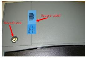
5. Close the touch screen display and secure the lock with a medium barrel key. Place a label seal vertically from the main section of the unit to the display.
