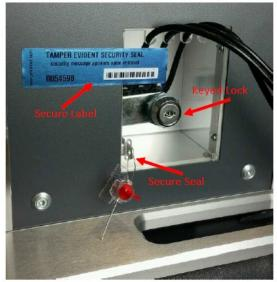
3. On the left side of the DS450, a clear access door protects the power switch, power cord, network port and USB port. The access door must be secured using the integrated key lock and a wire or padlock seal. A label seal must also be applied.
