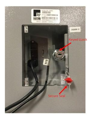
3. On the right side of the DS850, three clear access doors protect the USB ports. The access doors must be secured using the integrated key locks and wire or padlock seals.
