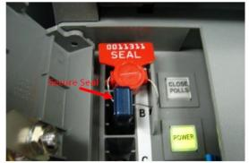
2. Close the access door and lock with a medium barrel key. Place a label seal.
