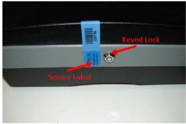
6. Place a second label seal on the seam where the top of the unit joins to the base.
