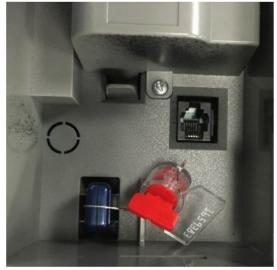
4. Ensure that the rear access door is locked with a medium barrel key and affix a label seal. The rear access door covers the backup USB flash drive.
