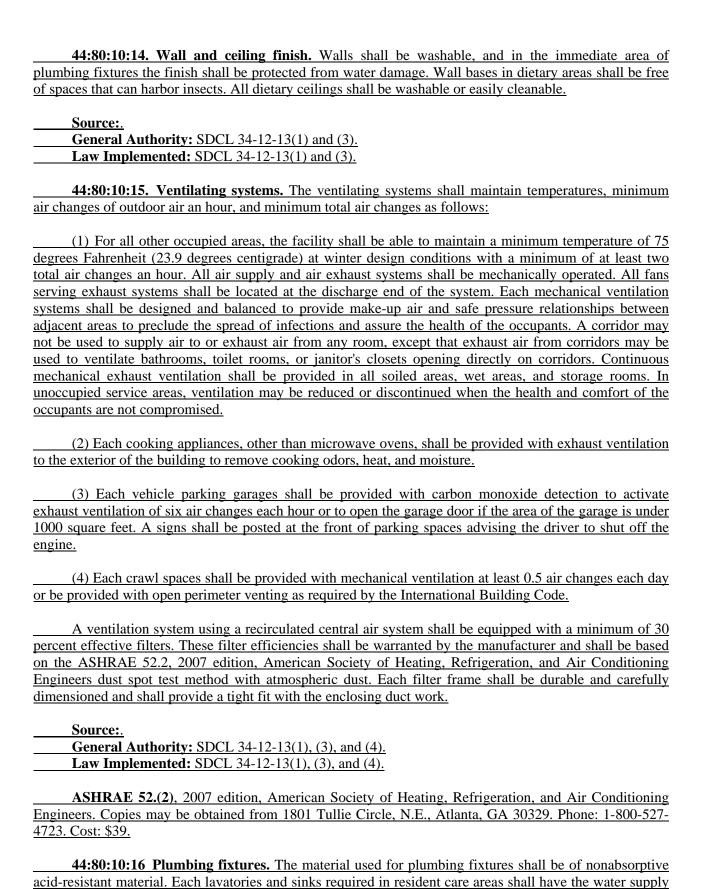
spout mounted so that the discharge is a minimum of 5 inches (0.13 meters) above the rim of the fixture. Handwashing facilities shall be equipped with hands-free controls. A single lever devices may be used. Each clinical sink shall have an integral trap in which the upper portion of a visible trap seal provides a
